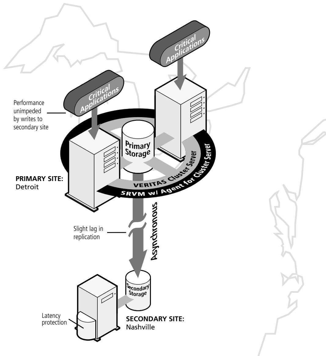
Figure 3. Company B – Asynchronous Replication to a Single Host
