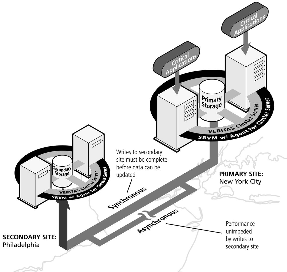
Figure 2. Company A – Synchronous Replication with Clustered Secondary
